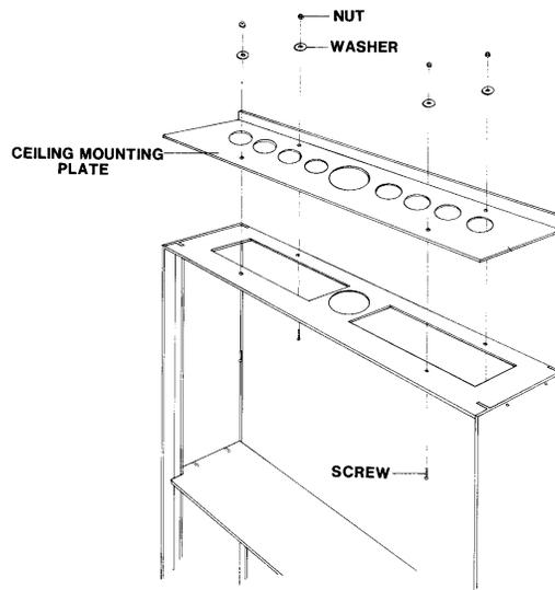
For those headwalls that include an adjustable base, once the headwall is in position, the adjustable feet at the bottom of the base can be screwed in or out until the top of the headwall is a snug fit to the ceiling mounting plate
